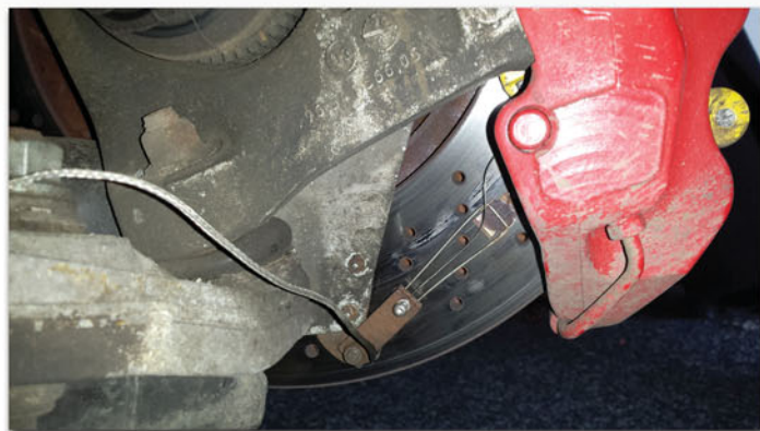
Above, rubbing thermocouple installation
