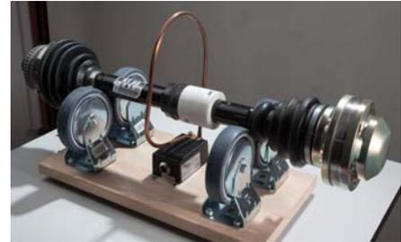
As data transmission of the D<sup>x</sup> is completely independent of power supply, the ring stator (or alternatively the inductive head) may be placed at any arbitrary place along the axle. Due to a built-in DC/DC converter in the sender, the quality of the power supply is of secondary importance.
