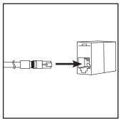
Connect Ethernet to the J3 Ethernet port cross coupler.
