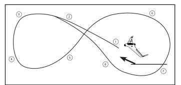
Aerial vehicles should be flown in figures of eight with some acceleration and braking and with the addition of climbs and dives. After 15-20mins system will be ready for use.
