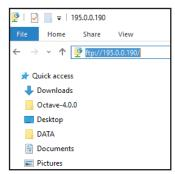
In the address bar, type "195.0.0.nn" where nn are the last two digits of the serial number.
