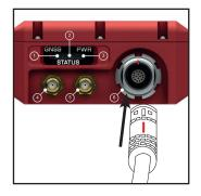
Align red marks on user cable and socket, then push to connect. Apply power (10-31 V d.c).
