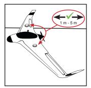
Antenna separation should be between 1 m and 5 m apart. Place the GNSS antennas on a metal parallel surface. Make sure the antennas have a ground plane to prevent GPS signal reflection.
