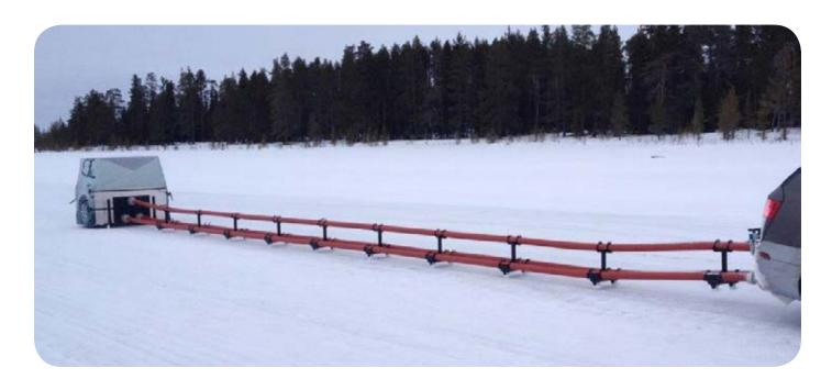
Moshon Data has developed the first Flex-Moshon EVT towing system for winter testing in the snow. Specifically adapted for winter AEB testing, the Flex-Moshon uses expertly designed skids instead of wheels which allows the towing system to glide across snow and ice.
