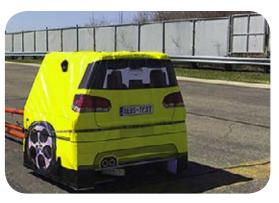
The MD-VT and MD-VT L (Large) is an inflatable, lower cost version of the official Euro NCAP Vehicle Target (EVT). It is designed to the same specifications as the Euro NCAP target and intended for development work. Being a cheaper substitute for the EVT means vehicle manufacturers and test facilities can purchase multiple vehicle targets and increase the number of tests.
