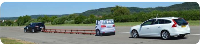
The Flex-Moshon towing system is designed to tow a balloon car during Autonomous Emergency Brake (AEB), Forward collision warning (FCW) and other ADAS tests.
