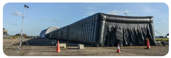
This is a unique 300ft (91m) long tunnel for testing ADAS sensors in the dark. Exclusively available from Moshon Data, the night vision tunnel provides interior light blocking to assist with the development of night vision assist technology. The tunnel consists of six 50' long connecting sections, five emergency exits/exit lights every 50' and three 5000 CFM exhaust fans to clear the air after every run through. The tunnel is suitable for AEB and VRU tests.
