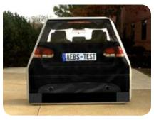
This target has been designed as a very low cost Demonstration Target, albeit constructed to a very high standard, the MD-SF has all the features of the more expensive models.
