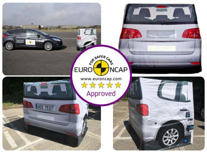
The Moshon Data EuroNCAP Vehicle Target (EVT) was developed to simulate the rear end of a standard production car and is suitable for RADAR, LiDAR and camera based systems.
