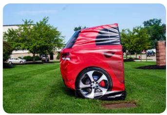
The MD-VT F is a lower cost, foam version of the official Euro NCAP Vehicle Target (EVT). It is designed to the same specifications as the Euro NCAP target and intended for development work. Being a cheaper substitute for the EVT means vehicle manufacturers and test facilities can purchase multiple vehicle targets and increase the number of tests.
